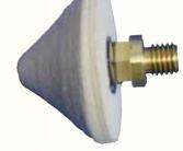
Felt Cones are an excellent choice for working bottles and inside curves. These cones are approximately 3" at base and 3" in height. The felt cones come with a 5/8"-11 male brass thread to fit a 5/8"-11 female thread. Use in combination with cerium oxide to achieve a high, optically-clear polish.
