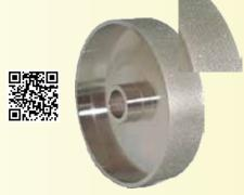
Covington's 6" and 8" Textured Grinding Wheels are excellent tools for pre-forming rough stone and glass material. The texturing allows for better sediment wash-out. These balanced, solid steel wheels, are nickel electroplated to provide superior bonding of diamonds and a long life.
