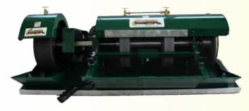
The #752 8" Silicon Carbide Grinder/Polisher comes with two 8" x 1-1/2" silicon carbide grinding wheels (100g & 220g), one 8" expandable drum, one 3" x 25-7/32" sanding belt (400g), and one 8" x 1"-14RH aluminum head with 8" leather disc, sample kit (polish powder, brush, dop sticks, and wax), instructions, and product guarantee.
