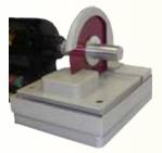
The Cab King Trim Saw Attachment features an 8" sintered blade, plastic blade guard, drip pan, pan support, splash guards, saw platform, and an additional platform for small rough stone. Spin off the right hand wheel and adapter, and spin on the special saw adapter with blade, set in place, and start cutting.
