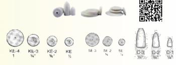
Felt Wheels and Points are used for buffing and polishing hard and soft metals, plastics, and painted surfaces. These are typically used in combination with a compound for desired effect and are excellent for polishing glass with cerium oxide. The wheels and points have a maximum speed rating of 15,000rpm.
