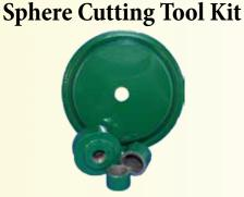
The Sphere Cutting Tool Kit will make spheres from 1-1/4" to 4" in size. Cups have a 1"-8RH threaded bore to fit horizontal lap arbors. This kit consists of a special splashguard and one (1) each: 1", 1-3/8", and 2-3/8" cutter cups. Sphere cutting on this unit is simple, just hold the rough sphere with a gloved hand and grind it on the proper size sphere cutter cup.
