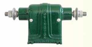
The **Two-Station Closed Arbor** is a low cost "build-your-own" style grinder/polisher. This versatile unit is designed to accept 6", 8", and 10" wheels. The arbor ships with two (2) nuts, 3" drive pulley, v-belt, and two (2) sets of 3" diameter flanges. The split housing, with a closed center, connects using two bolts. Two bearings are set on the shaft with two set screws. This arbor can
