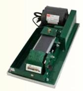
The **#460** Horizontal Wet Belt Sander is designed for grinding flat surfaces such as tiles. This sander uses 3" x 25-7/32" sanding belts and comes complete with a 1/3hp motor mounted on a rustproof aluminum-topped Lam-I-Cushion base, a water valve and spray nozzle for water supply hook up, 3" x 6" backing plate, instructions, and product guarantee. This machine ships with the motor attached, ready to plug in and operate.
