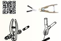
The **Split Plier** is designed for use with the #2 Vise & Power Feed 1/2"-13 threaded rod. The 6-1/4" long bronze pliers assembly comes with a spring, pivot stud, lock nut and two (2) each fiber washer and metal wear washer. The **Split Clip** is designed for use with the 1100 & 1500 series saws. The 3" long spring loaded split clip comes with a 5/16"-24 split nut in its jaws.
