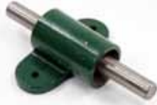
CAR110 - $40.00 5/8" Smooth Shaft 6-1/4" Overall Length 5/8" x 1-3/4" Pulley End 3" Mounting Hole Spacing 1/4" Hole Diameter
