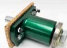
Newly Redesigned! 1100 Replacement Arbor CAR14R - $69.00 5/8"-18RHT 1-3/4" Pulley End 5-1/2" Over All Length 3" Mounting Hole Spacing 1/4" Hole Diameter 1/8" Max. Space between 2" Flanges 6061 Aircraft Aluminum with two separated bearings for stability!
