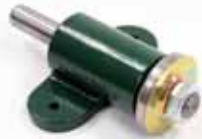
CAR13R - $50.00 5/8"-18RHT 5-1/2" Overall Length 5/8" x 1-3/4" Pulley End 3" Mounting Hole Spacing 1/4" Hole Diameter 1/8" Max. Space between 2" Flanges
